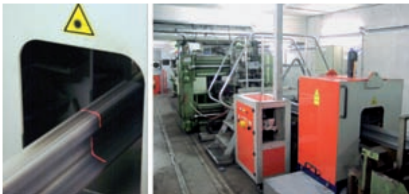
10 Links: Profilmessung an durchlaufenden Schienen, rechts: Ansicht der Profilmessanlage im Schienenprüfzentrum Left: profile measurement of rails running through the measuring unit, right: view of the profile measurement system at the rail inspection center Foto: TSTG Schienen Technik
